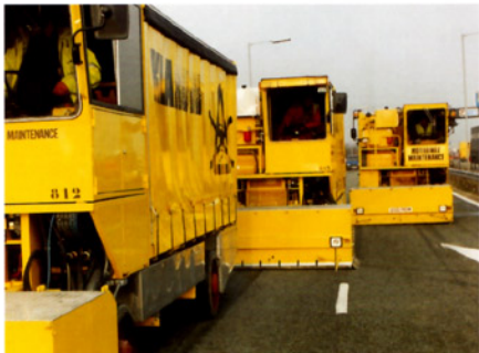
A Klarus K190 retexturing machine in action
