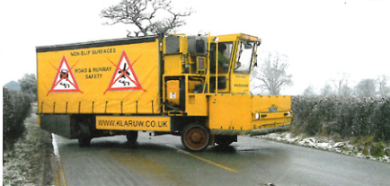
Moving works: Four-wheel-drive and twin-axle steering make the machine manoeuvrable. Light 'StopGo' traffic control is generally sufficient during operation.
