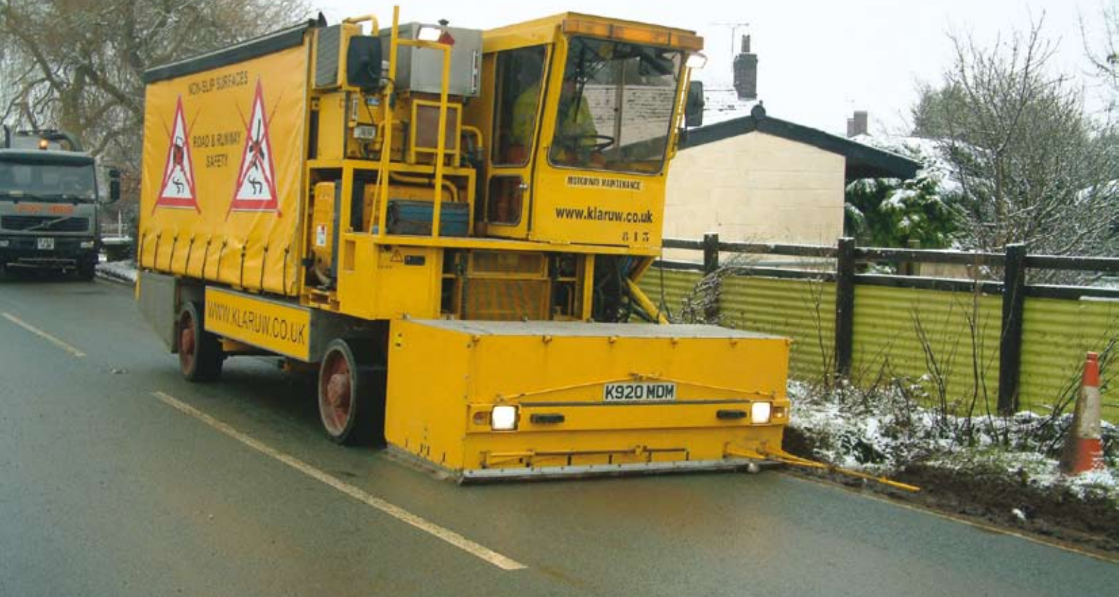
(Above) Retexturing processes are generally not plant and process-intensive, producing a smaller carbon footprint. Traffic management is less onerous and there is less disruption to motorists.
